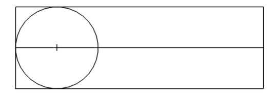
4. From the centre of the Circle, measure 25mm back towards the left edge of the piece. Mark it and make a Punch mark. This and the remaining Punch marks will be used for drilling so can be a bit heavier than the first one you did.
