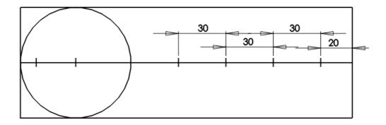
6. From the Centre Line measure and mark 15mm up the left edge of the piece. Also from the Centre Line measure and mark 15mm up the right edge. Join these two marks with your Scriber and Ruler.
