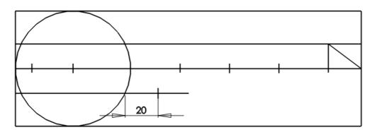
10. Now using your Ruler and Scriber, draw any key tooth form that you like from the mark made in the last step to the end of the Centre Line on the right side of the piece. When that is done you are finished the marking out.
