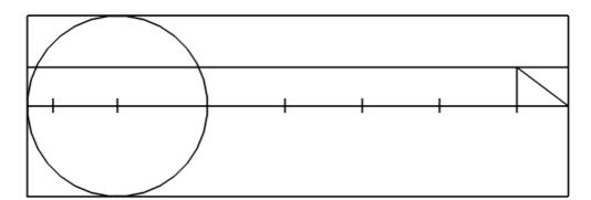
8. From the Centre Line, measure and mark 15mm down the left edge of the piece. T-Square a line about half way across the piece.
