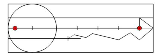
12. Next, using a 5mm Drill Bit, drill the remaining 4 holes as shown below. You then tap these 4 holes with an M6 Tap. Hold the piece of metal flat in a Bench Vice while you are tapping and make sure the Tap is perpendicular to the holes. If you are making the Key Holder from Steel you should use some Tapping Compound or Cutting Fluid.
