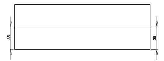
2. From the left edge, along the Centre Line, measure and mark 35mm. Make a light Punch mark here, enough to seat the point of a Dividers.
