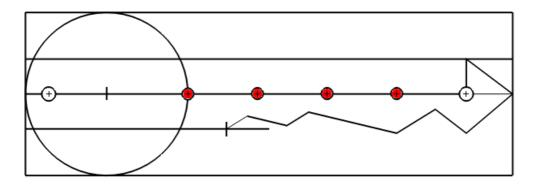
13. Next you will have to cut out the shape using a Hacksaw. Below are some images showing some possible cuts. Think about how you might cut it out as you may come up with a better way. Cut off as much as you can with the Hacksaw without going over the lines of the Key shape.
