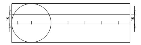
7. Using your T-Square and Scriber, from the Punch mark on the Centre Line that is 20mm in from the right edge of the piece, scribe a line up to the 15mm line that you drew in the last step. Then join this point back to the right edge of the Centre Line, as shown below.
